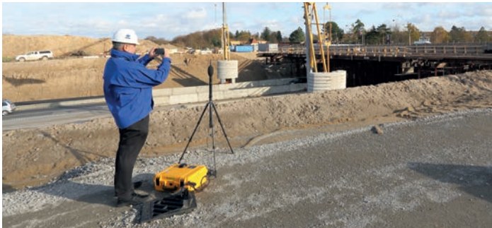
Fig. 9 A portable NMT used independently from a central software system
