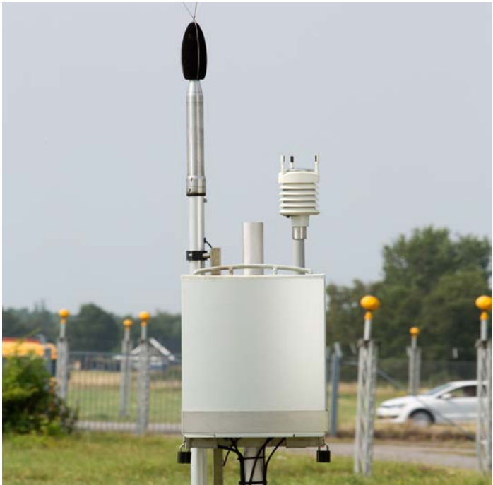
Fig. 2 Permanent NMT mounted on a pole
